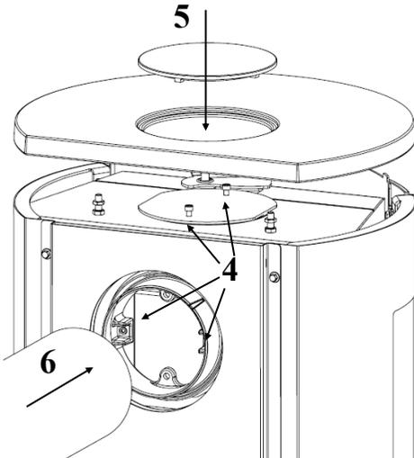
1. Cut the discs out in both back plate layers.
